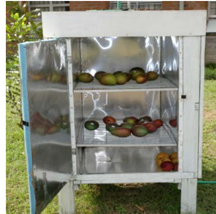
Fig.3 The near infrared reflecting (NIR) charcoal cooler loaded with mango fruits
