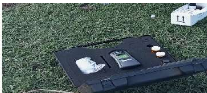
Plate 3.2: Turbidimeter used to measure turbidity in the field
