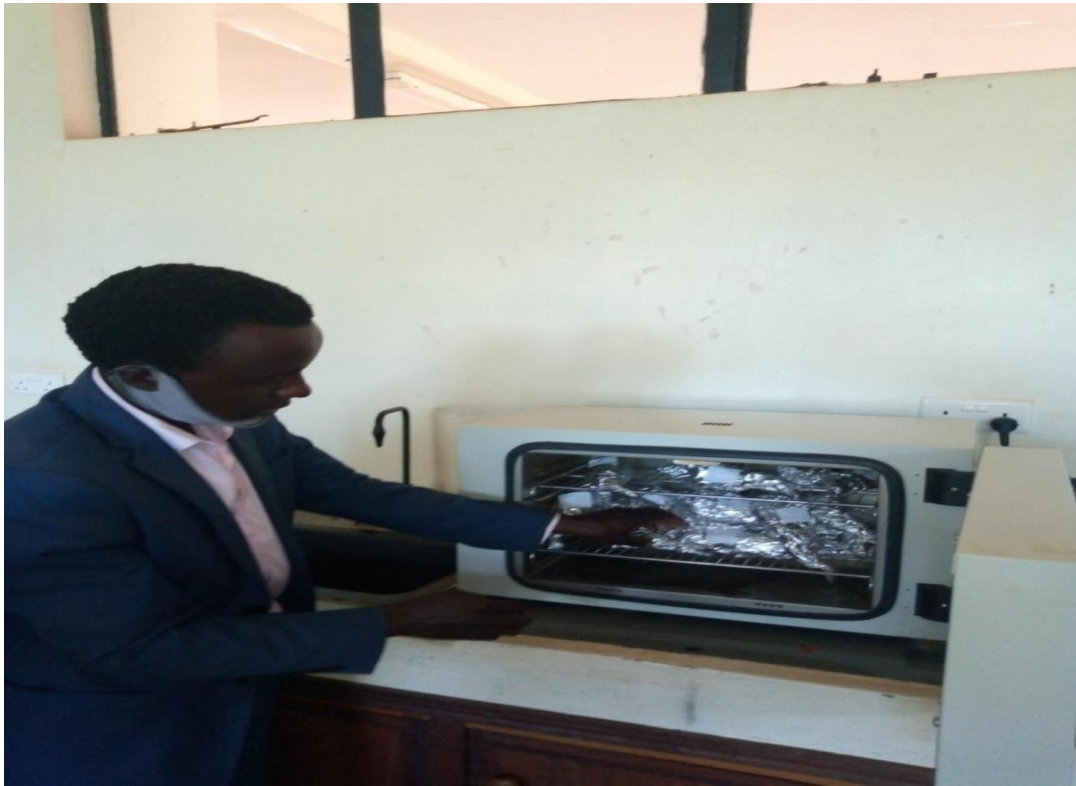
Figure 4.2: Tile Powder Samples Being Fed into the Hot Air Oven for Drying at South Eastern Kenya University.
