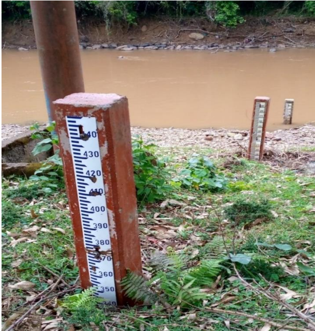
Plate 3.1: Staff gauges installed in Kipsonoi Sub basin RGS 1JF08 on 16/08/2020 (Source: Koech, 2021)
