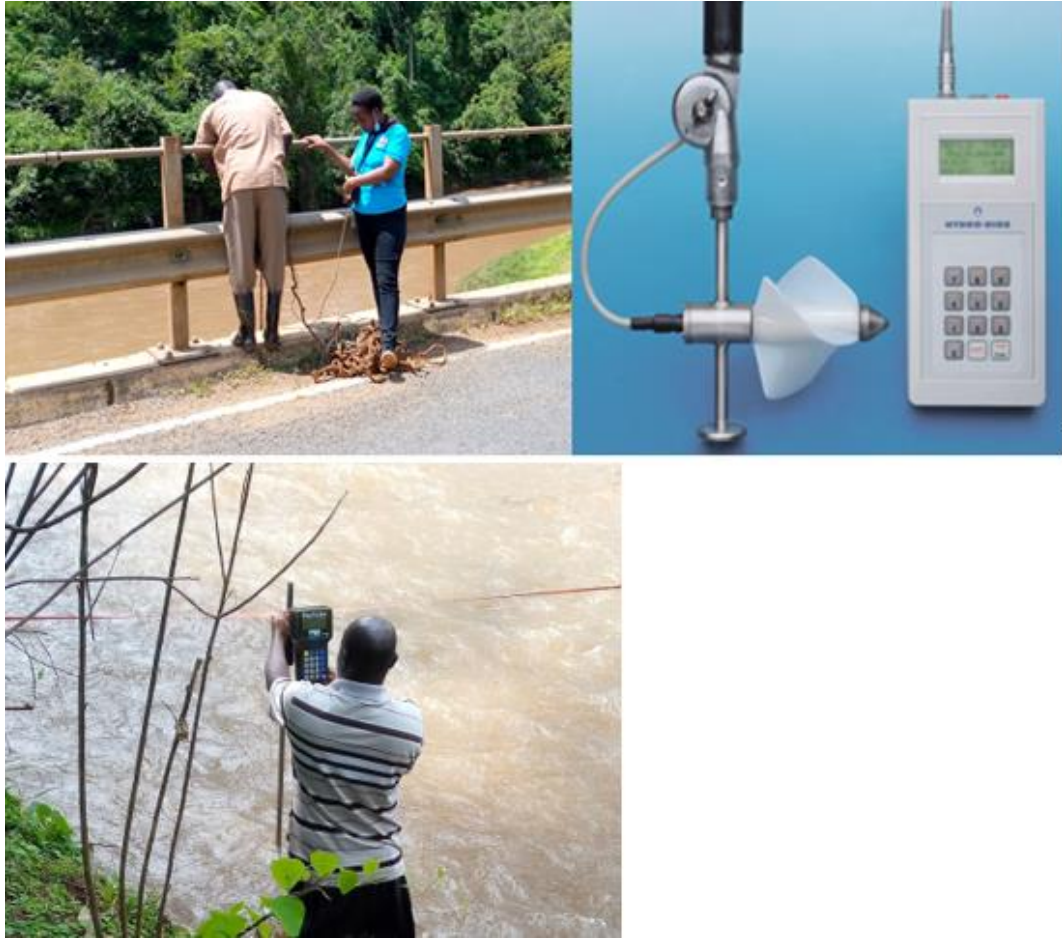
Plate 3.1: Velocity measurements in Kipsonoi sub basin on 18/10/2020 (Source: Koech, 2021)
