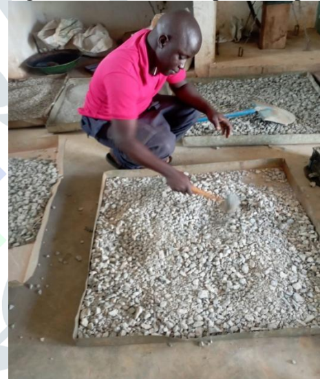
concrete debris being crushed
