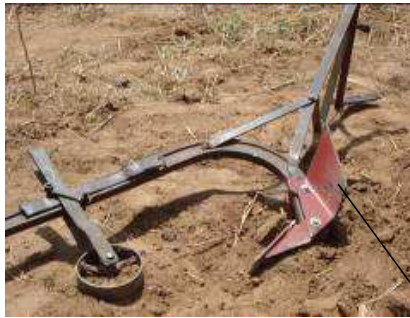
Fig 2. Ripper fitted in exchange for sub-soiler and wide furrows made after widening the 6inch deep narrow furrow left by sub-soiling.
