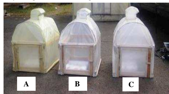
Fig. 1 Plates showing the experimental set-up of the model solar tent dryers
