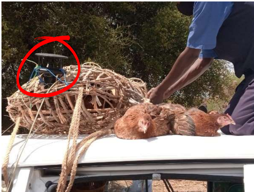
Plate 3.3: Placement of Anemometer to determine air speed
