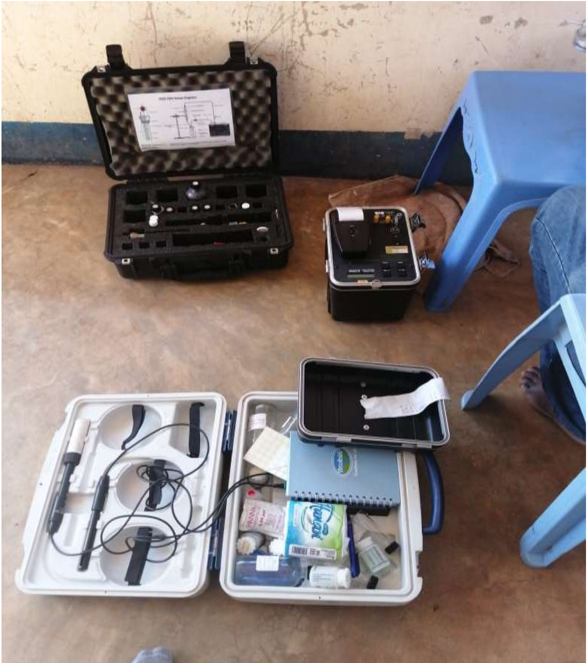
Assembling RAD 7 Alpha detector in the field for Radon measurements
