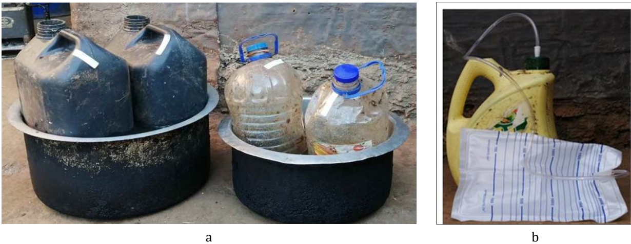
Figure 1 A set-up of (a) biogas production at the thermophilic condition (b) Volumetric biogas measurement setup
