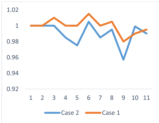
Figure 3.0: Voltage profile in MODED with RE Vs Bus Position
