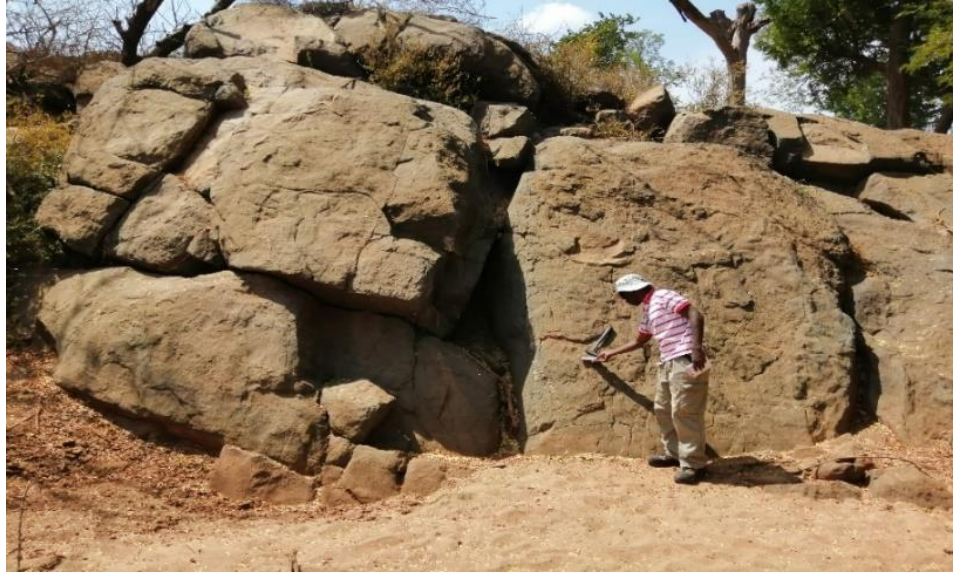
Plate 3. 2: Measurement of joint structures in Meta-pyroxenite rocks of Mwitika area.
