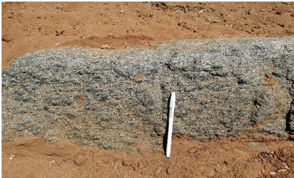
Plate 4. 20: A lineated and protomylonitized Meta-pyroxenite occurring in Mavia mailu area showing a preferred parallel orientation (UTM: 426317/9832830). The lineation trend at 29^{\circ} NE and plunges at 50^{\circ} .
