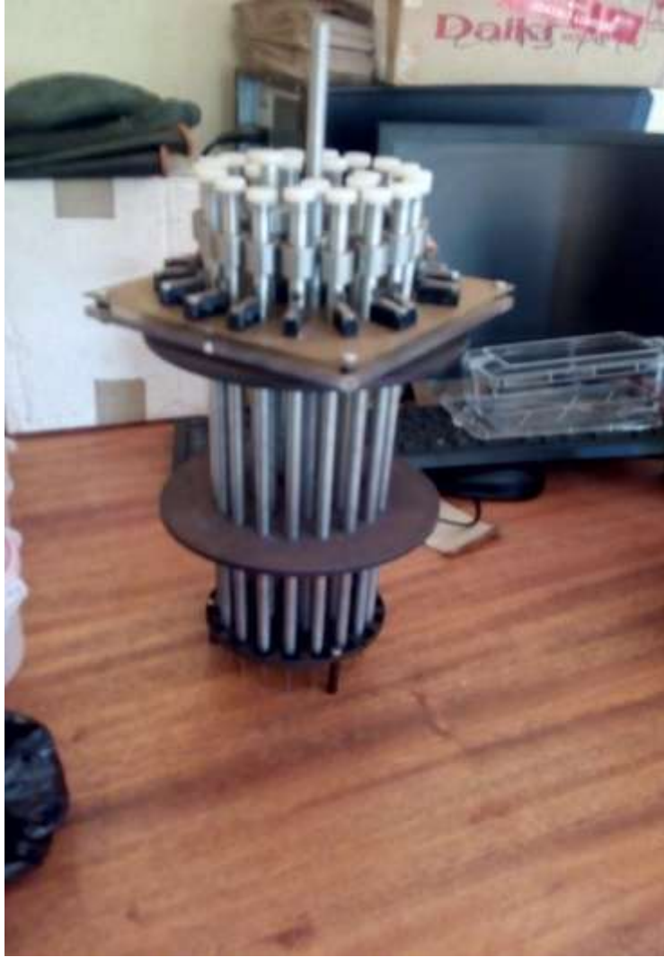
Plate1: Mattson Cooker with Cooking rank with plungers dropped down indicating the switch was on. (Photo by Josephine Syanda)
