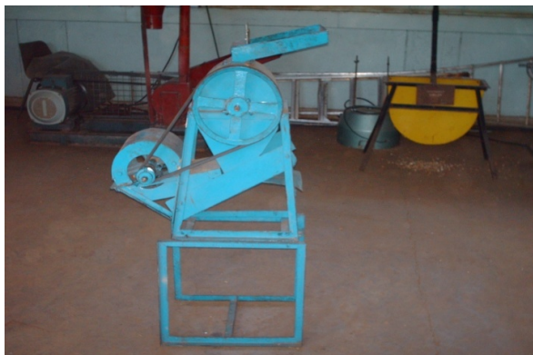
Figure 2. Wooden beater decorticator.
