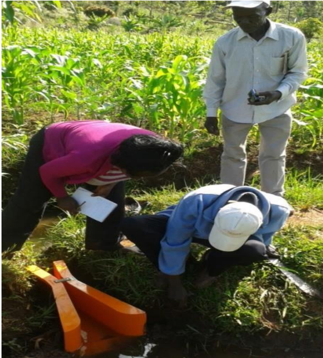
Figure 4.3 : Measuring water abstraction by open channel in Thiba River using parshall flume: Source Kasuni (2016).
