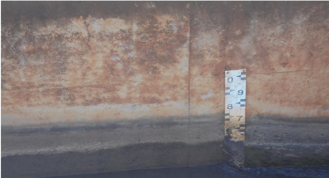
Figure 4.4 : Staff gauge contributing to data located at checkpoint I at Nyamidi headrace used for flow measurements. Source: Kasuni (2016).
