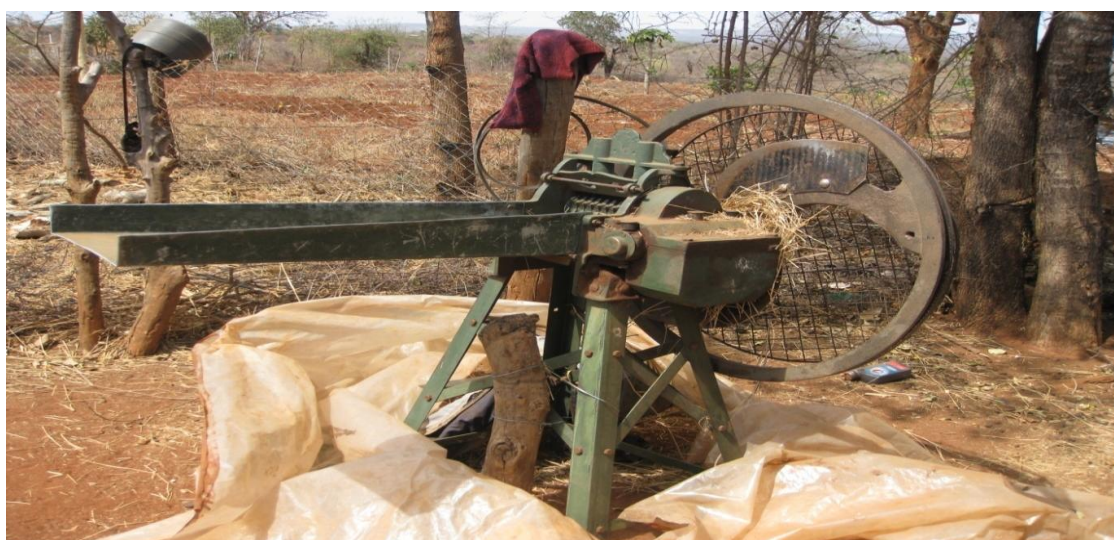
Figure 4.9: Chaff-cutter for chopping feedstuffs
