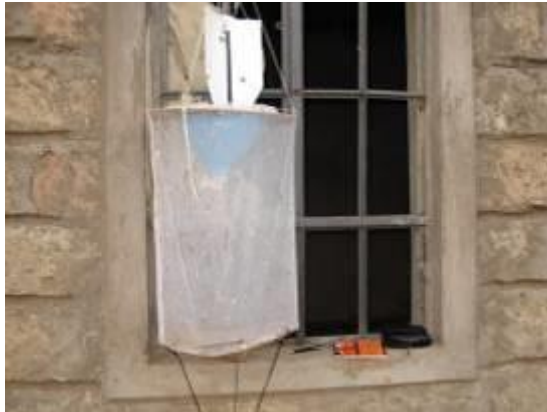
Plate 3.4: Sample of the moth light trap with 6 watt actinic tube suspended over a butterfly net.
