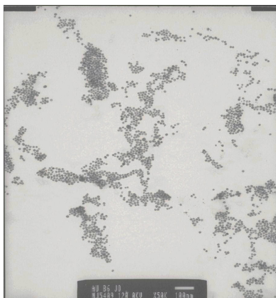
Figure 2. TEM image of colloidal gold nanoparticles.
