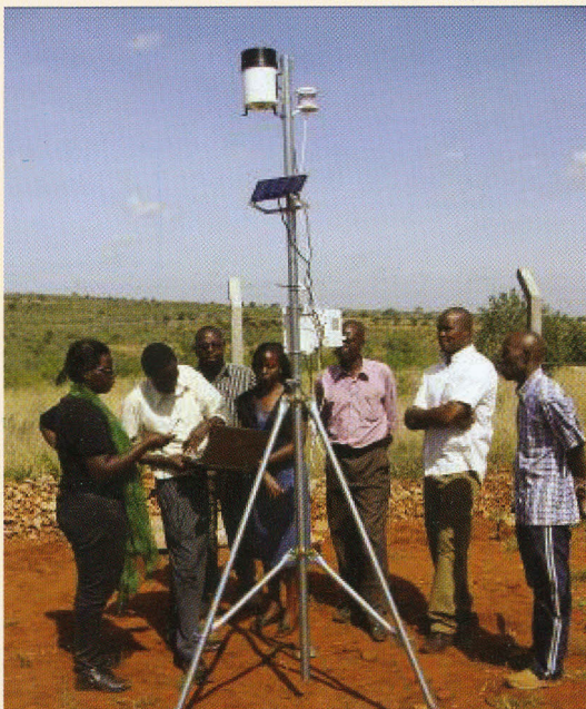
Mini automatic weather station being installed by researchers from ICIPE through the School of Earth Sciences at the University.
