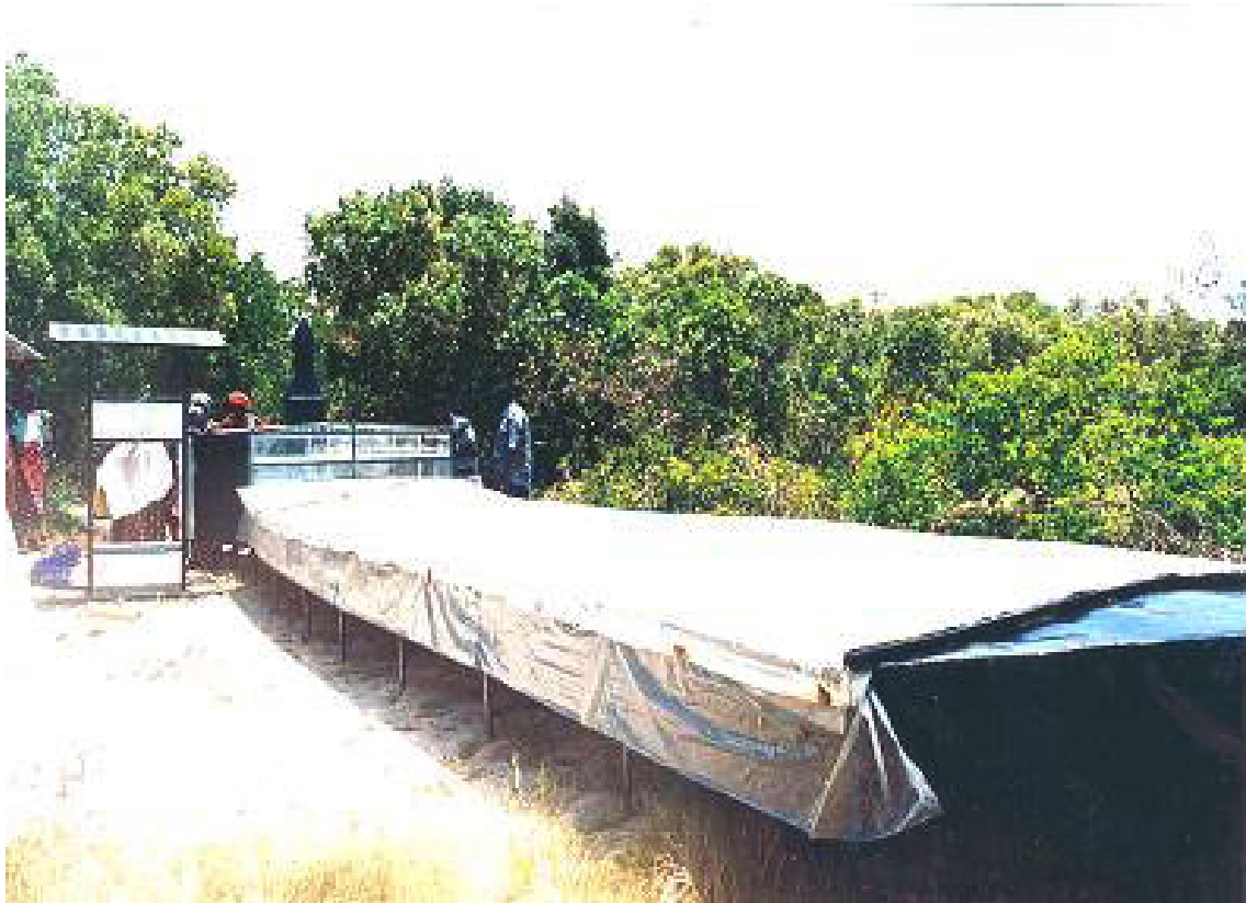
Figure 1. View of designed tunnel dryer
