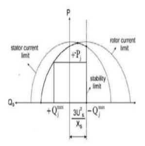
Fig 2:DFIG Capability Limits Curve[20]
