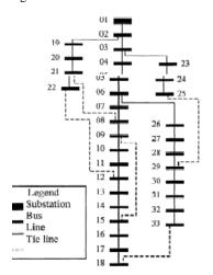
Figure 3:IEEE 33 Bus Radial Distribution System
