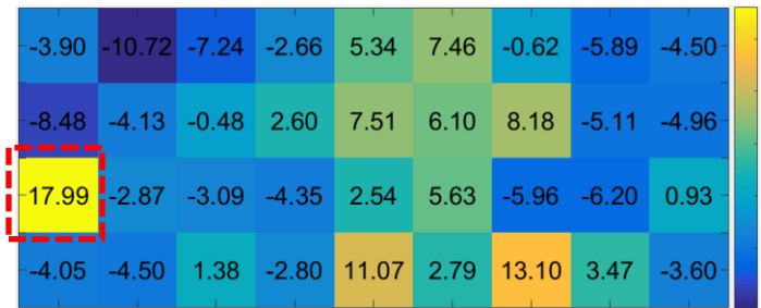
Fig. 5. Cell voltage deviation from mean (22 V, 5 A), scale from -11 mV to 18 mV, mean of 0.609 V
