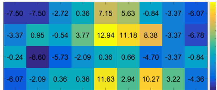
Fig. 4. Cell voltage deviation from mean (18.9 V, 1 A), scale from -8.6 mV to 12.94 mV, mean of 0.524 V
