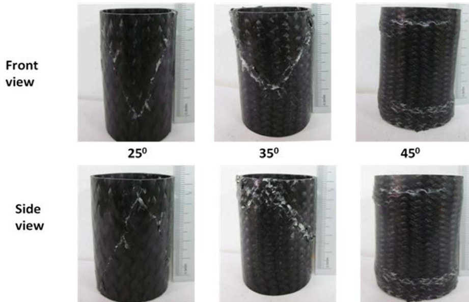
FIG. 15. Damage morphology of samples with different braiding angle. [Color figure can be viewed at wileyonlinelibrary.com ]
