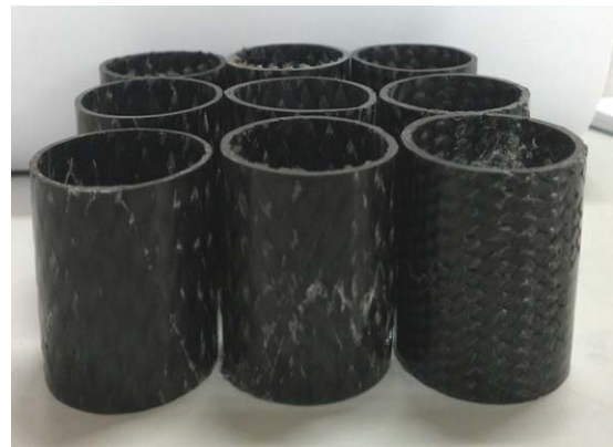
FIG. 4. Samples of same height but different braiding angle. [Color figure can be viewed at wileyonlinelibrary.com]
