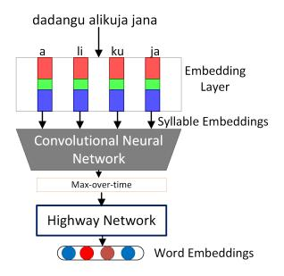
**Figure 1.** The Architecture of WEFSE demonstrating how the Swahili word *alikuja* is split into its respective syllables and subsequent composition of the embeddings. The convolutional layer provides the composition function to generate the word embeddings.
